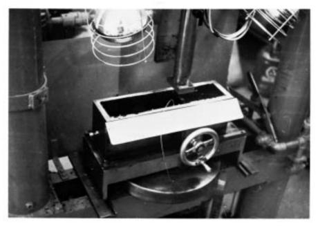
FIG. 1 Beam Mold Assembly in California Kneading Compactor
