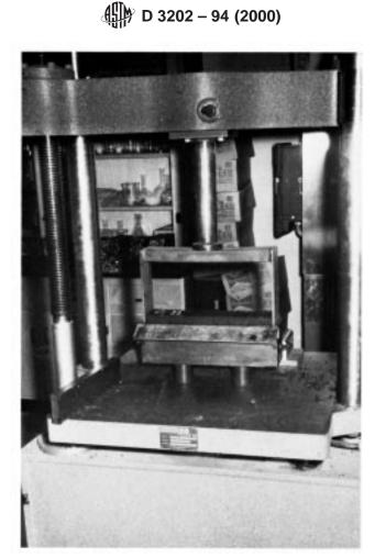
FIG. 2 Beam Extraction Assembly
